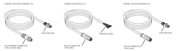
Refer to Gocator 2000 I/O Connector (page 302) for pinout details. Refer to Parts and Accessories (page 325) for cordset lengths and part numbers. Contact LMI for information on creating cordsets with customized length and connector orientation. The maximum cordset length is 60m.
