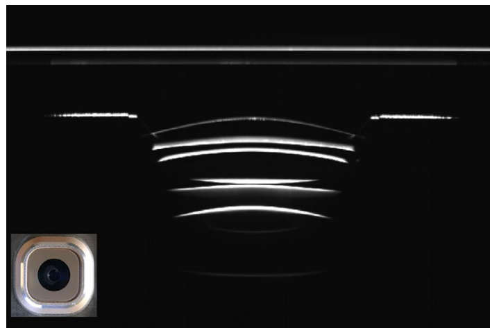
Smartphone camera structure visualized by using FocalSpec Line Confocal Sensor LCI1201. In addition to dimensional measurements, particles and delaminated camera optics can be identified.
