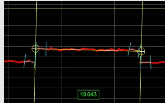
Measures the width of a strip.
