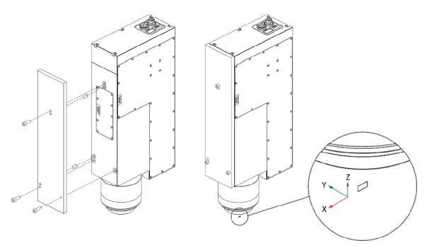
Optionally, use the two 6mm alignment pin holes (depth 6mm) to help align the plate and sensor holes. Note the indicated orientations of the coordinate system in the images above. Note that mounting is identical for the G4010 model.
