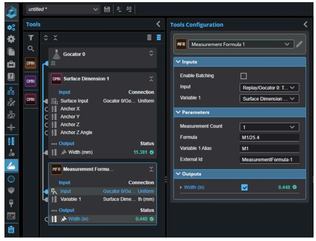
In this example, a Measurement Formula tool is used to convert a width measurement from a Surface Dimension tool from millimeter units to inches by using the formula "M1/25.4".
