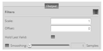
Scale and offset adjustments can be applied using both the Script tool and the Measurement Formula tool. Here is an image demonstrating the use of the Measurement Formula tool for this
