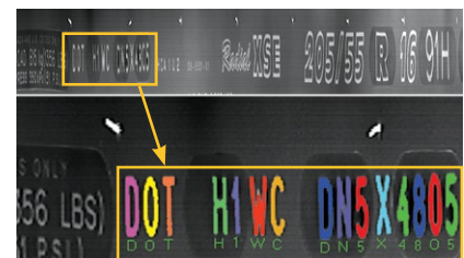
DOT-code is generated simultaneously from height data
